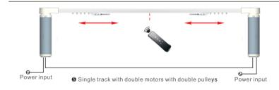
RF control + pulse switch - separate control and group control solution
